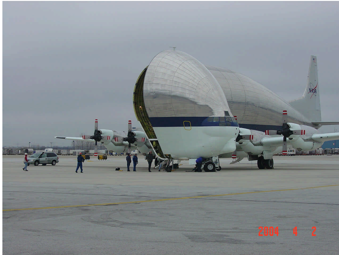
Super Guppy off load operations at Philadelphia Airport Nose is open
