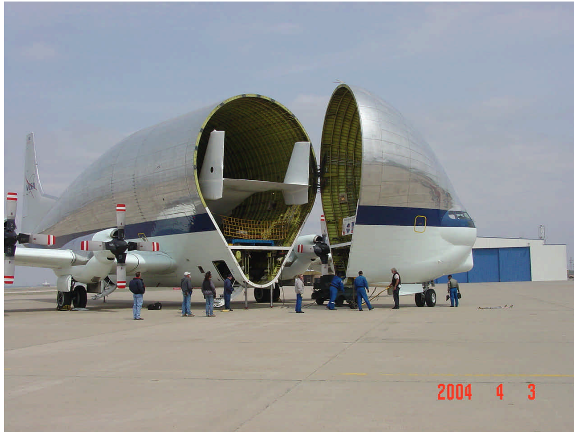
Super Guppy off load operations at Amarillo Airport Nose is open
