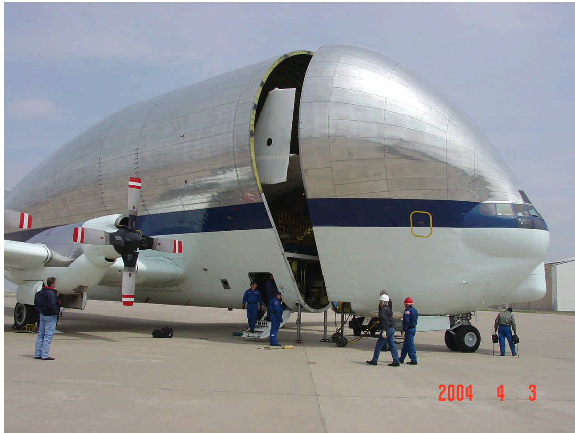
Super Guppy off load operations at Amarillo Airport Nose is being open
