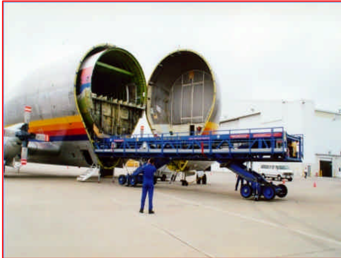
Section 46 Offload Operation Waco, TX
