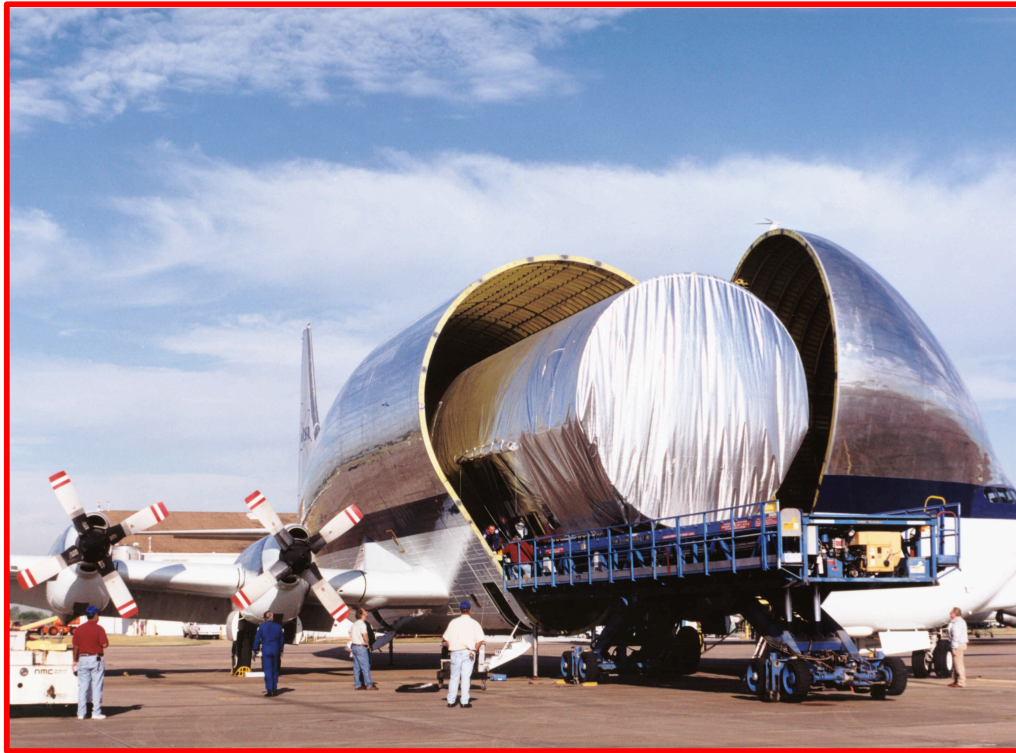
P3/P4 STA Offload Operation Ellington Field, TX
